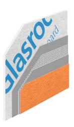
Direct Render finishing is used for the construction of external walls in which the board is exposed to the external environment. The render should be a compatible basecoat mortar using a reinforcement mesh. Finish the system using an acrylic or siloxane-based topcoat.
