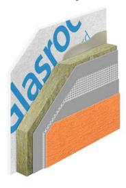
ETICS or EIFS Systems are used for construction of external walls in which the board is exposed to the outside. A continuous external insulating system is then adhesively / mechanically fixed to the Glasroc® X board. The complete system is then finished using an acrylic or siloxane-based topcoat.
